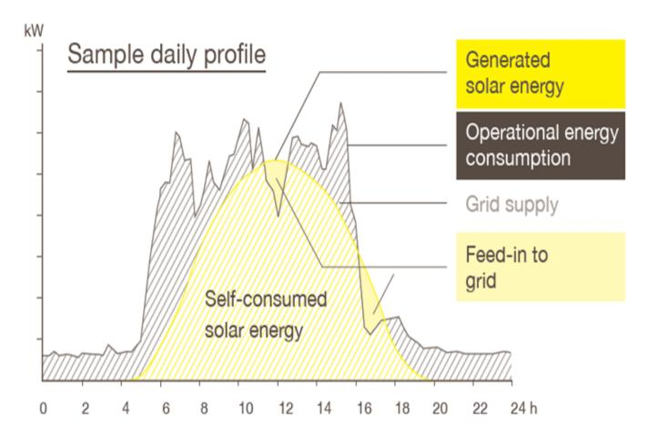
Sample daily load profile for a plastic manufacturing company with self-consumption from PV (Kraftwerk 2015)
