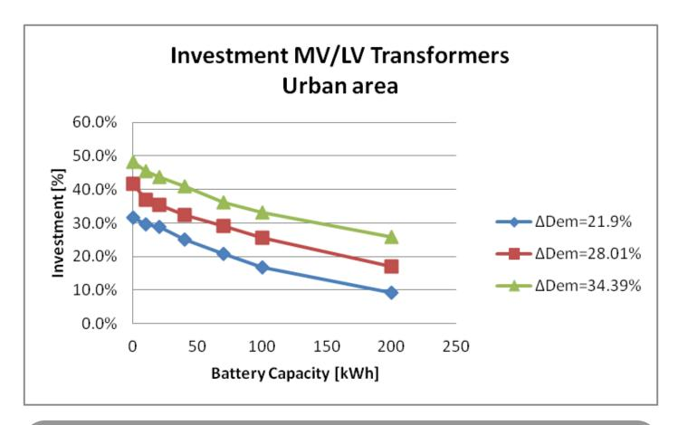
The required investment as a percentage of the existing assets depends on the storage capacity connected at each transformer
